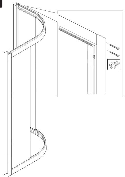
(a) Install the screws to both sides to secure the assembly.
