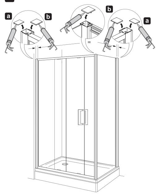
(a) Fit the plastic covers to the top of the extrusions.
