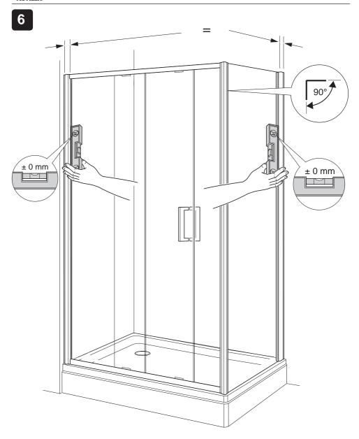
(a) Centralise the door frame within the wall channels, making sure that the door frame is square.
