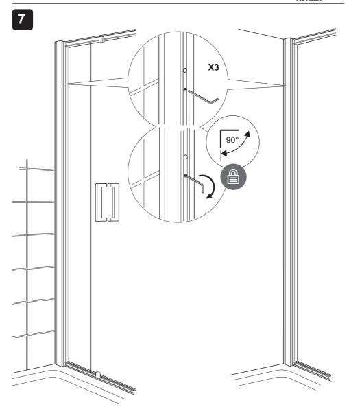
(a) Using the 3.0 mm hexagonal wrench (supplied), turn through 90° clockwise to lock the door frame, corner post and side panel in position.
