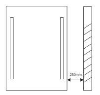
Ensure the sensor are positioned at least 250mm away from any solid surface including walls.
