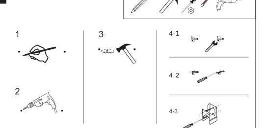
Measure the distance between the two brackets, mark the distance on the wall, check the marks are level, drill the holes, insert the wall plugs and fix according to 4-1, 4-2 or 4-3
