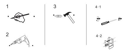
Measure the distance between the two brackets, mark the distance on the wall, check the marks are level, drill the holes, insert the wall plugs and either 4–1 insert screw or 4–2 fix bracket.
