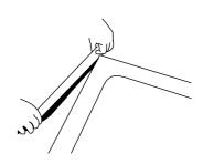
Wipe the surfaces clean where the strip will be attached first with a clean damp cloth, allow to dry and then wipe with the IPA wipe supplied in the kit.
