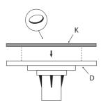
Attach the Circular Adhesive Pads (3) to the under-side of all the Circular Base Plates (3) by removing the backing paper from one side ONLY of the Adhesive Pads (3), centralise and push firmly into position.
