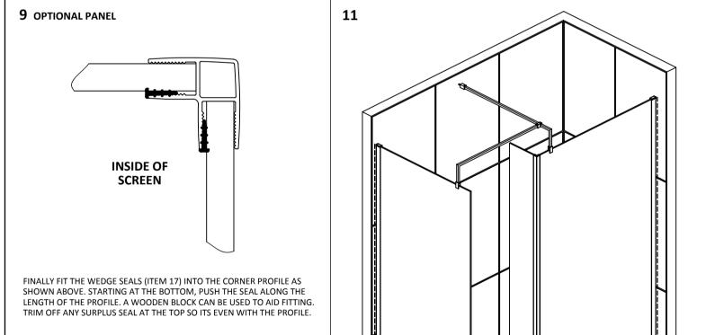
EXTERNALLY SILICONE SEAL THE WALL PROFILE WHERE IT MEETS THE WALL AND ALONG THE BOTTOM OF THE GLASS. ALL IN A CONTINUOUS BEAD.
