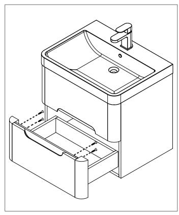
1. Open drawer and remove four fixing screws holding the existing insert. Keep screws safe for re-use.
