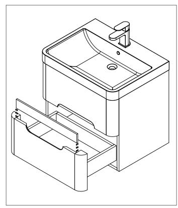
2. Remove insert and replace with selected colour insert
