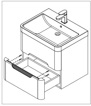
3. Use the four screws to re-attached the new colour insert.
