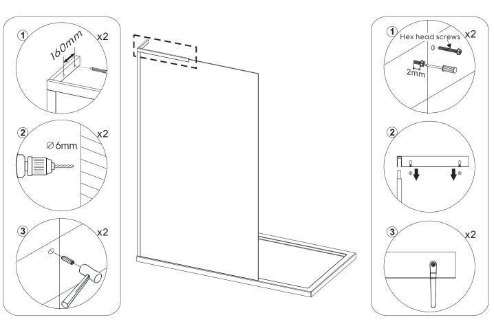
STEP 8 FITTING THE SUPPORT BAR SYSTEM SEALS AND CAPS
