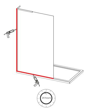
Allow 24 hours for silicone to dry before use. Silicone on the outside edge only
