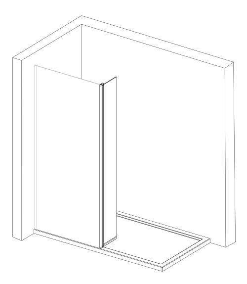
Install the main Wet Room Glass Panel before fitting the Flipper Panel
