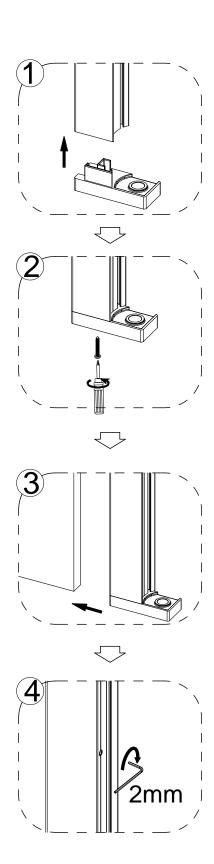
Step 2 - Install glue strip to the bottem of the glass Atlach the up base to the profile and fix it with screws.
