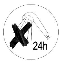
Allow 24 hours for silicone to dry before use . Silicone on the outside edge only
