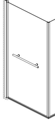
EXTERNALLY SILICONE SEAL THE WALL PROFILE WHERE IT MEETS THE WALL AND ALONG THE BOTTOM OF THE PROFILE AND MOULDING UP TO THE LARGE BOTTOM SEAL. ILLUSTRATED BELOW. ENSURE THAT YOU DON'T SILICONE THE LARGE BOTTOM SEAL.
