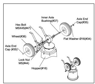
Insert the axle tube into the bushing and make sure they are tight.
