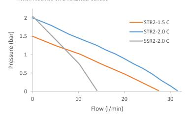
Pump performance at 230V with 2m inlet head
