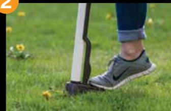
Press the pedal with your foot to the ground. Then remove your foot and pull the shaft.
