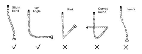
Important: Failure to follow these guidelines may result in poor performance and damage to the flexible connecting pipes.
