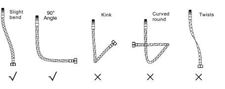
Important: Failure to follow these guidelines may result in poor performance and damage to the flexible connecting pipes.
