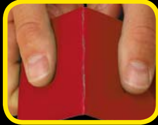
Brand X Cracks and flakes when bent
